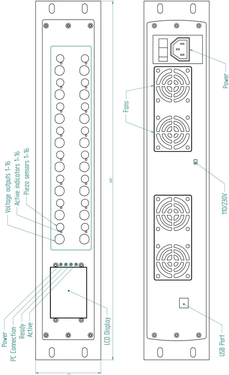
Figure 1: Front and rear panels of PAQ-16000D
