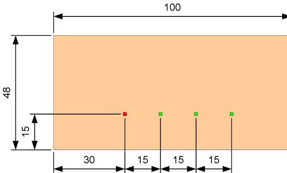
Figure 5: Arrangement of the piezoelements on the structure
